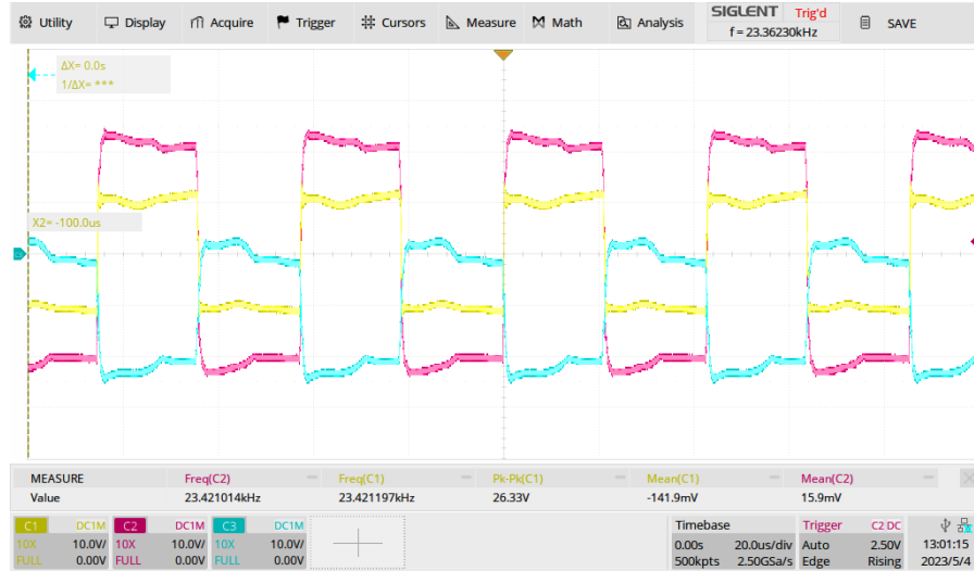
Figure 19: The differential output of the H-bridge when switching \sim 10V .
