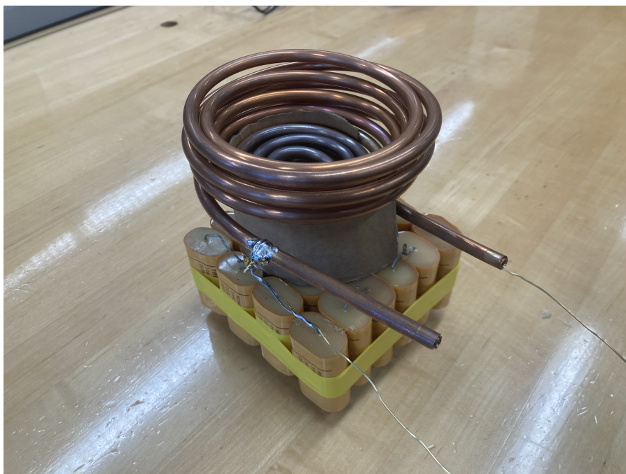
Figure 15: The parallel LC circuit, consisting of the work coil and the resonant capacitor bank.
